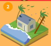
Category 2 96-110 MPH Extremely dangerous winds will cause extensive damage: Well-constructed framed homes could sustain major roof and siding damage. Many shallowly rooted trees will be snapped or uprooted and block numerous roads. Near-total power loss is expected with outages that could last from several days to weeks.
