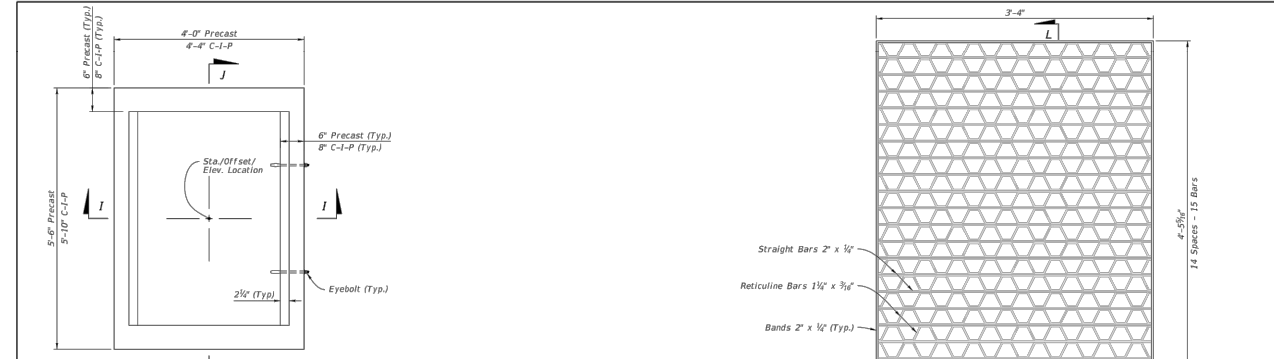
TYPE D - DIMENSIONAL, REINFORCING, AND STEEL GRATE DETAILS
